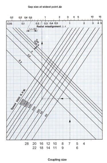
The permissible angular misalignment  $\Delta \not \leq$  is given as a measurable linear dimension  $\Delta$  b.
