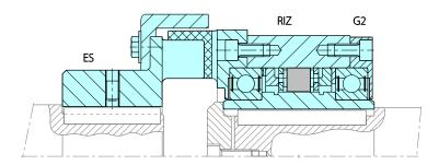
Fig. 12: RIZ..ESG2 installation example
