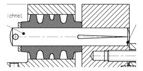
Fig. 11 Grooved pins with EL sizes 2 to 4
