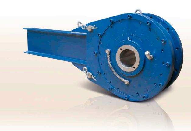
Backstops type RDBR-E are directly mounted on the drive shaft, e.g. of heavy duty conveyer belts, mixing drum drives and chain conveyors, when torque limiting / load sharing or the release function is required.
