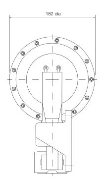
Weight (caliper and thruster) - 10.5kg (thruster only) - 4kg Volume displacement of thruster at 4mm retraction is 5ml
