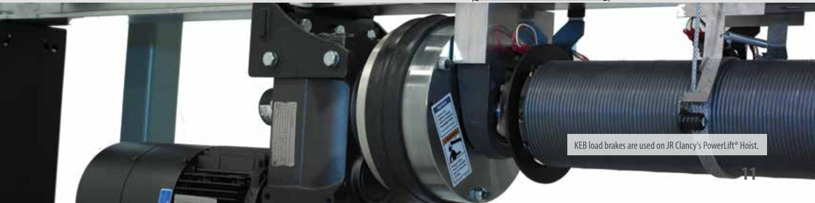
KEB load brakes are used on JR Clancy's PowerLift® Hoist.
