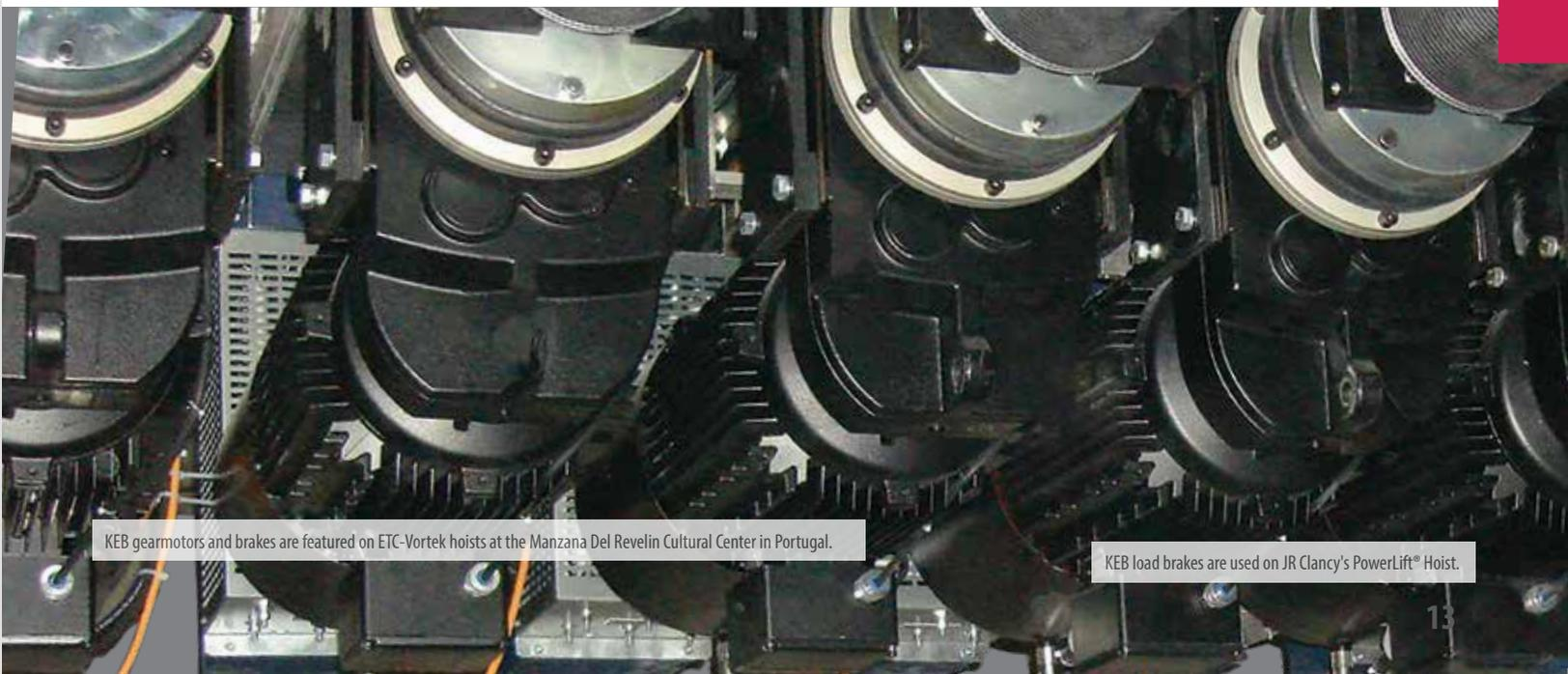
KEB gearmotors and brakes are featured on ETC-Vortek hoists at the Manzanera Del Revelin Cultural Center in Portugal.
