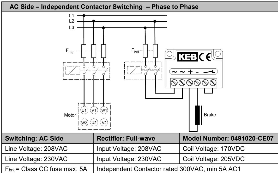
Figure 23 Rectifier Wiring AC Side Switching - Independent Contactor Switching - Phase to Phase
