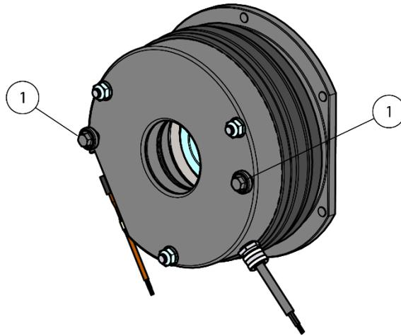
Figure 13 Bolt Removal
