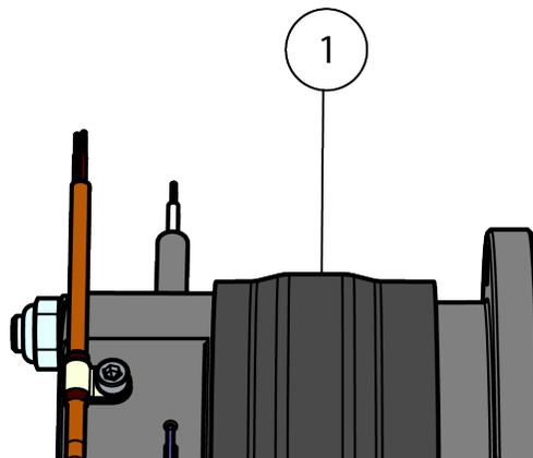
Figure 12 Dust Protection Ring
