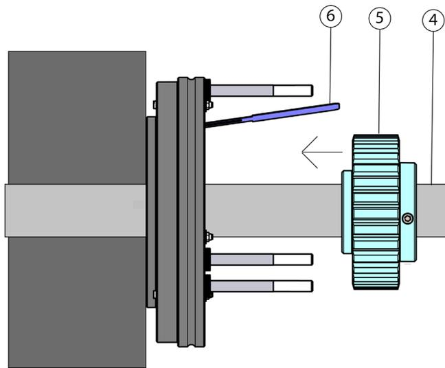
Figure 8 Hub Installation
