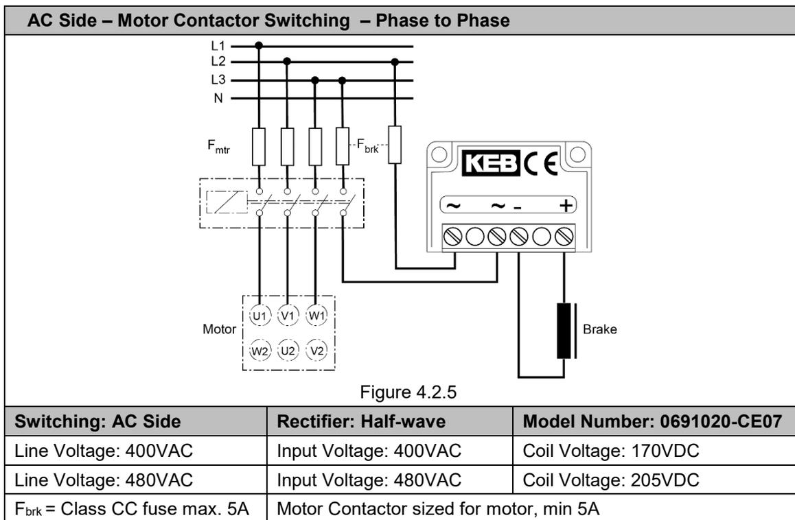
Figure 24 Rectifier Wiring AC Side Switching - Motor Contactor Switching - Phase to Phase
