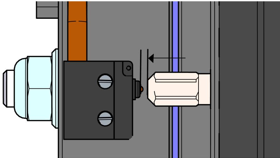
*Figure 21 Plunger Adjustment*
