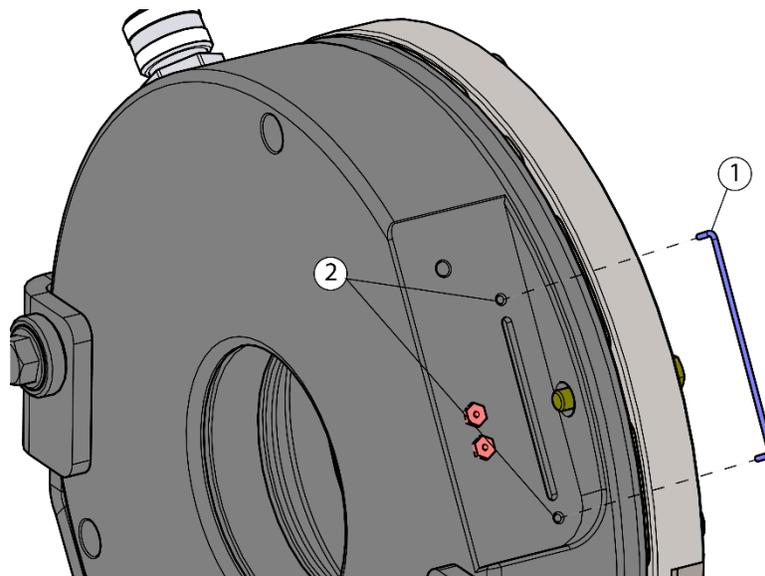
*Figure 16 Anti-rotation Wire Attachment*
