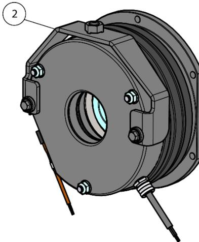
Figure 14 Hand Release Yoke Attachment
