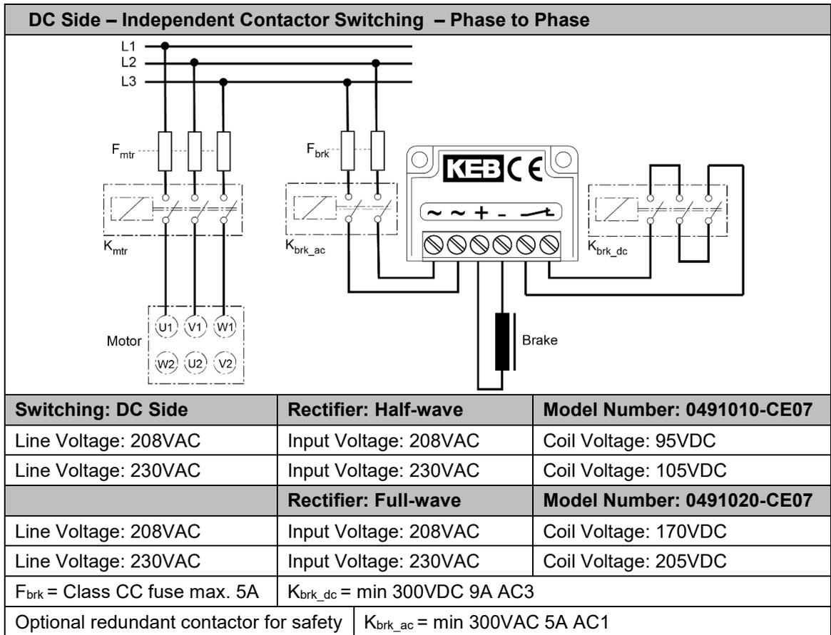
Figure 25 Rectifier Wiring DC Side Switching - Independent Contactor Switching - Phase to Phase
