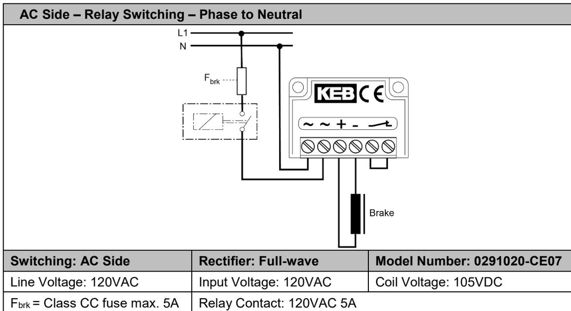
*Figure 22 Rectifier Wiring AC Side Switching - Relay Switching - Phase to Neutral*
