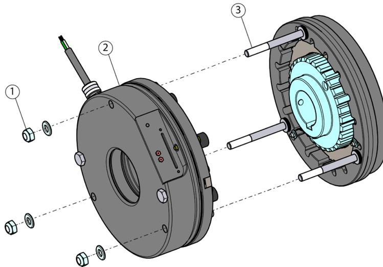
Figure 5 Magnet Removal
