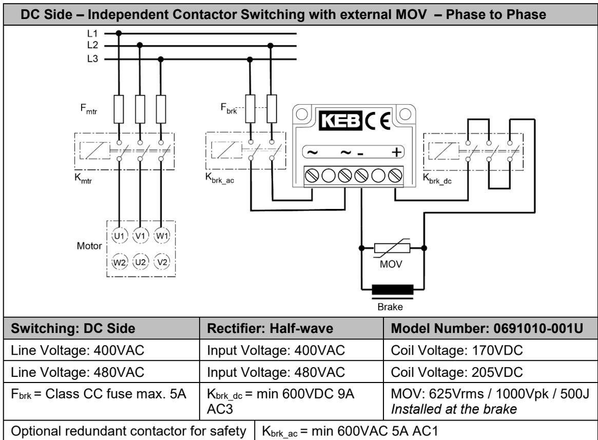
Figure 26 Rectifier Wiring DC Side Switching - Independent Contactor Switching with External MOV - Phase to Phase
