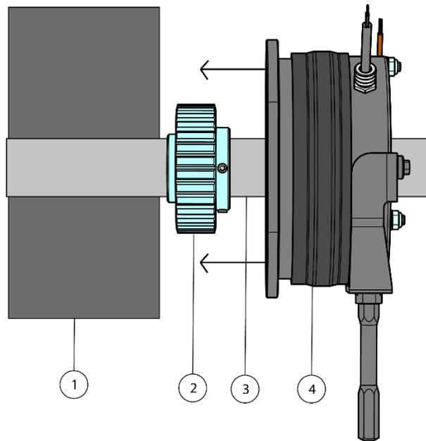
Figure 4 Brake Assembly Installation
