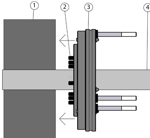
Figure 7 Brake Assembly Installation
