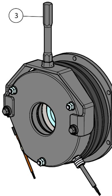
Figure 15 Hand Release Lever Attachment
