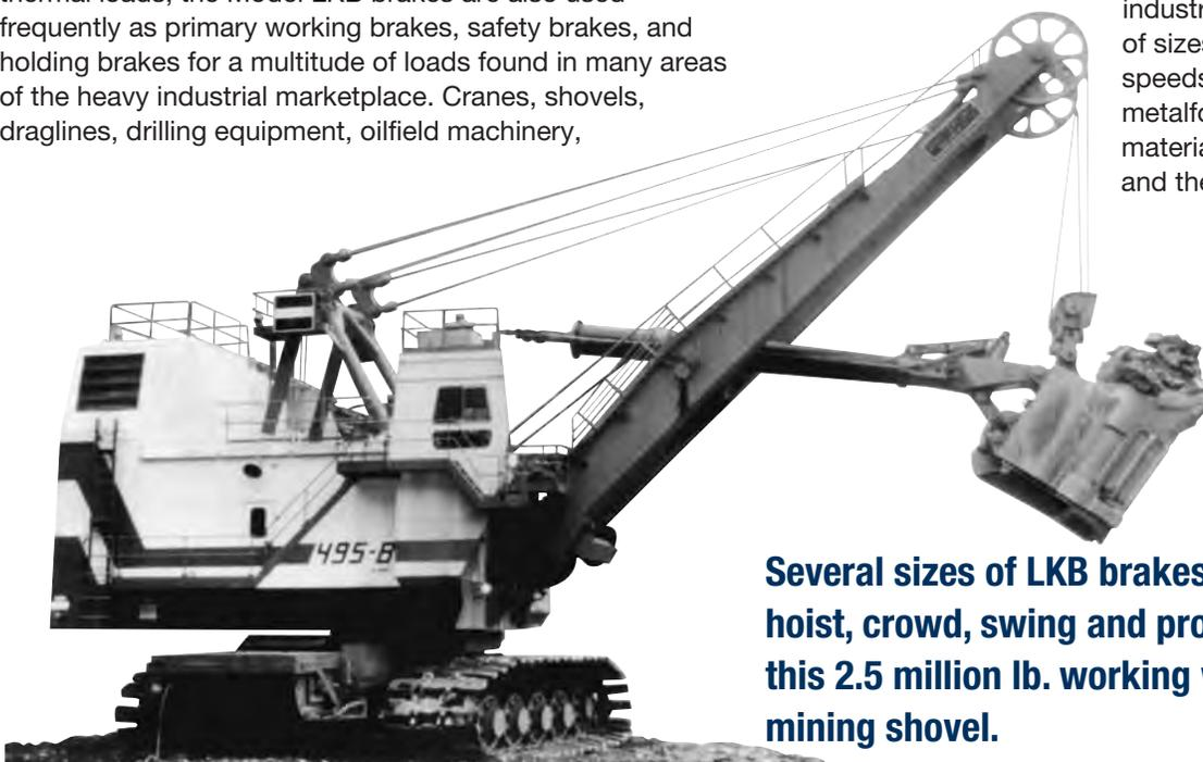
**Several sizes of LKB brakes are used on the hoist, crowd, swing and propel functions for this 2.5 million lb. working weight electric mining shovel.**
